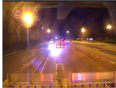
Figure 6: Example of false alarm due to the aperture problem. The optical flow vector are normal to the light beam edge giving completely wrong results.
